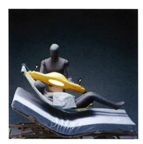
Just like being carried up gently in both arms, SASUKE is capable of lifting the care receiver directly off the bed from underneath the sheet, while bearing its whole weight.
